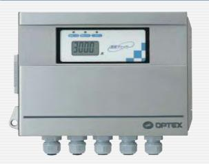
As well as the turbidity indication, this Transmitter can indicate signal output response time, alarm level setting, and so on. You can control the turbidity utilizing its functions fully.
