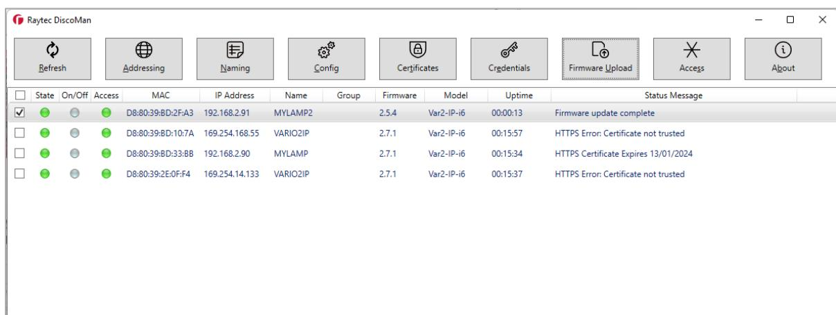
Click 'Refresh' and you should see the firmware column now displays the new firmware version next to the lamp. The lamp must restart at the end of this process so you will see this reflected in the *Uptime* column.
